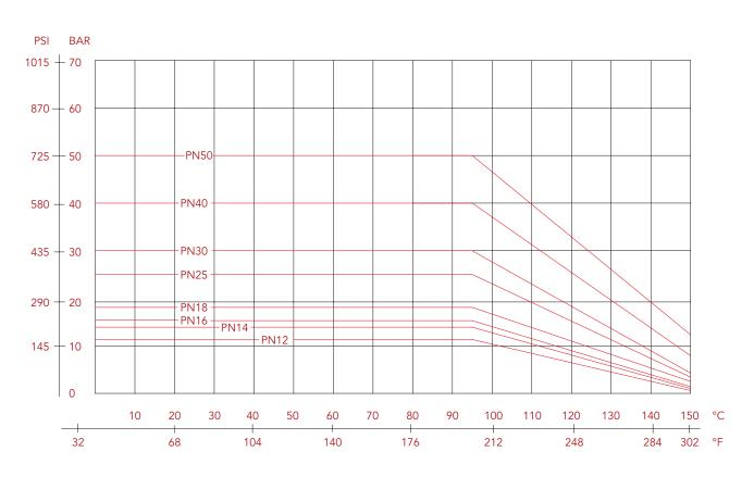
The values shown by the dropping lines state the maximum limit of employment of the valves. The shown valves are approximate.
