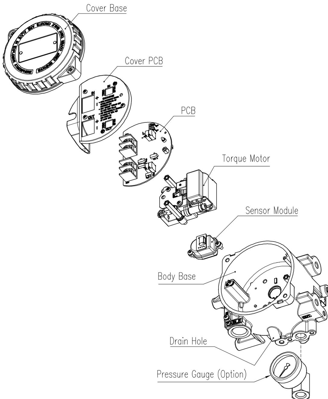
Fig. 2-1: exploded view
