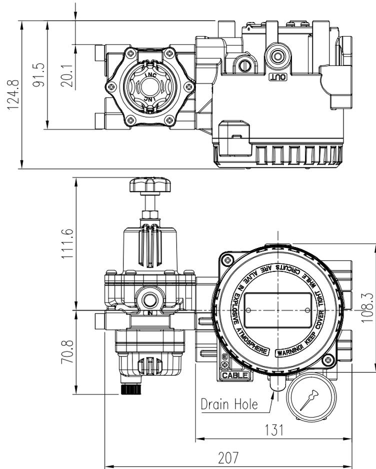
Fig. 2-3: YT-930 + Air filter regulator(YT-200) + Pressure gauge
