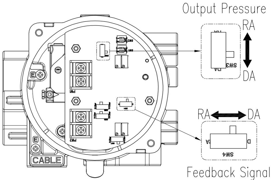
Fig. 6-2: DA, RA setting (without PCB cover)
